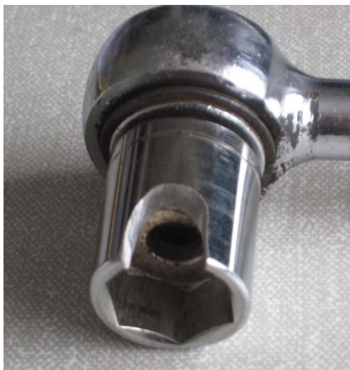
Detail of a modified 17mm socket
