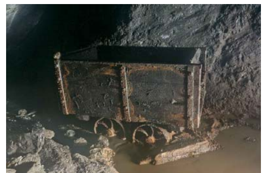
Wooden tub in the tramming level
